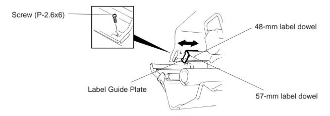
**NOTE:** Ensure that the label guide plate aligns with the dowel.
